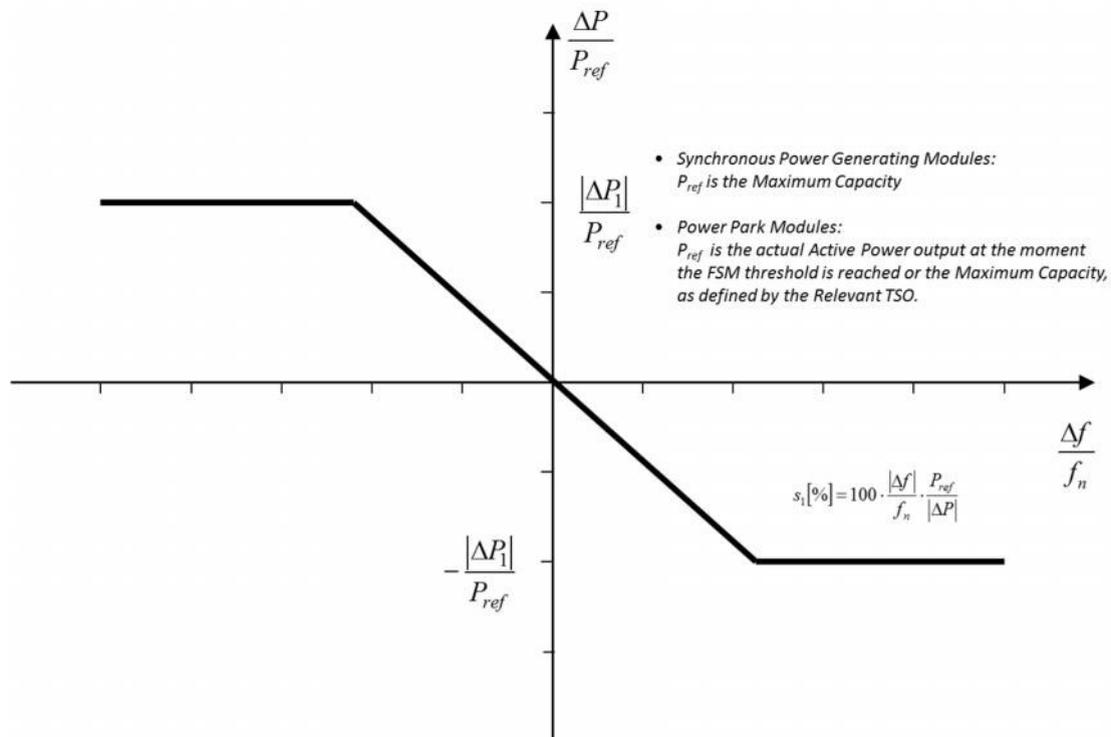
$P_{ref}$  is the reference active power to which  $\Delta P$  is related.  $\Delta P$  is the change in active power output from the power-generating module.  $f_n$  is the nominal frequency (50 Hz) in the network and  $\Delta f$  is the frequency deviation in the network.
