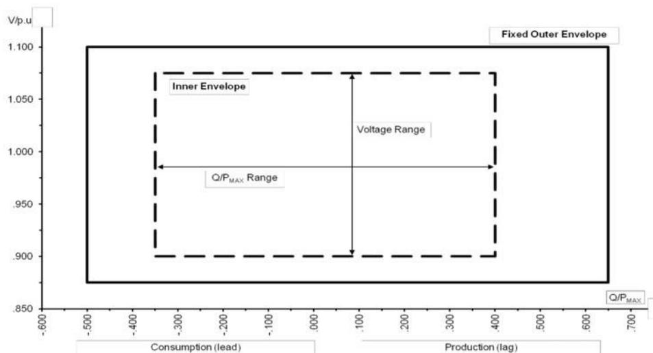
The diagram represents boundaries of a U-Q/P<sub>max</sub>-profile by the voltage at the connection point, expressed by the ratio of its actual value and its reference 1 pu value, against the ratio of the reactive power (Q) and the maximum capacity (P<sub>max</sub>). The position, size and shape of the inner envelope are indicative.
