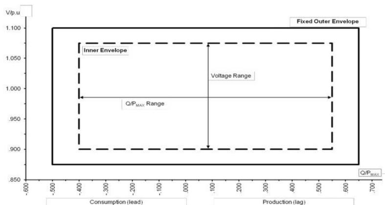
The diagram represents boundaries of a U-Q/Pmax-profile by the voltage at the connection point, expressed by the ratio of its actual value and the reference 1 pu value, against the ratio of the reactive power (Q) and the maximum capacity (Pmax). The position, size and shape of the inner envelope are indicative.
