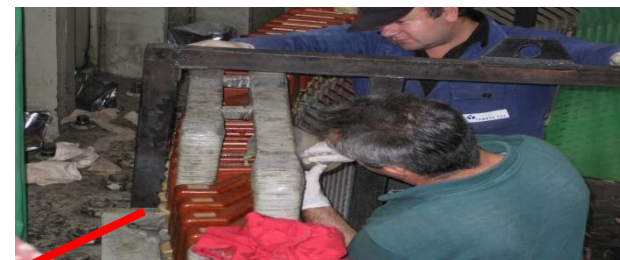
Stator repair & tests
